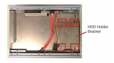
3. Use screw drvier to remove the screws. Keep the screws safely for later use.
